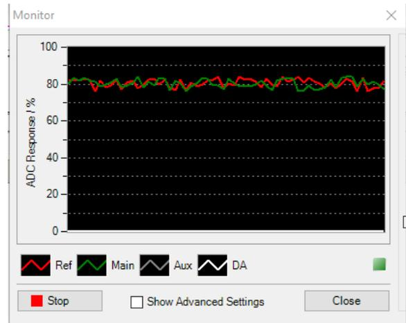
The manual setup panel will be visible along with the live display. This allows the user to change wavelength and read signals for both 0% and 100% for each channel.
