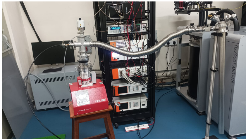
Figure 9: Helium gas line attached to Turbo pump and Suction pipe is attached with Inner (vacuum) sample space
