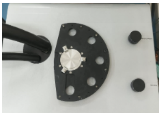
Figure 4: Remove these 3 screws
