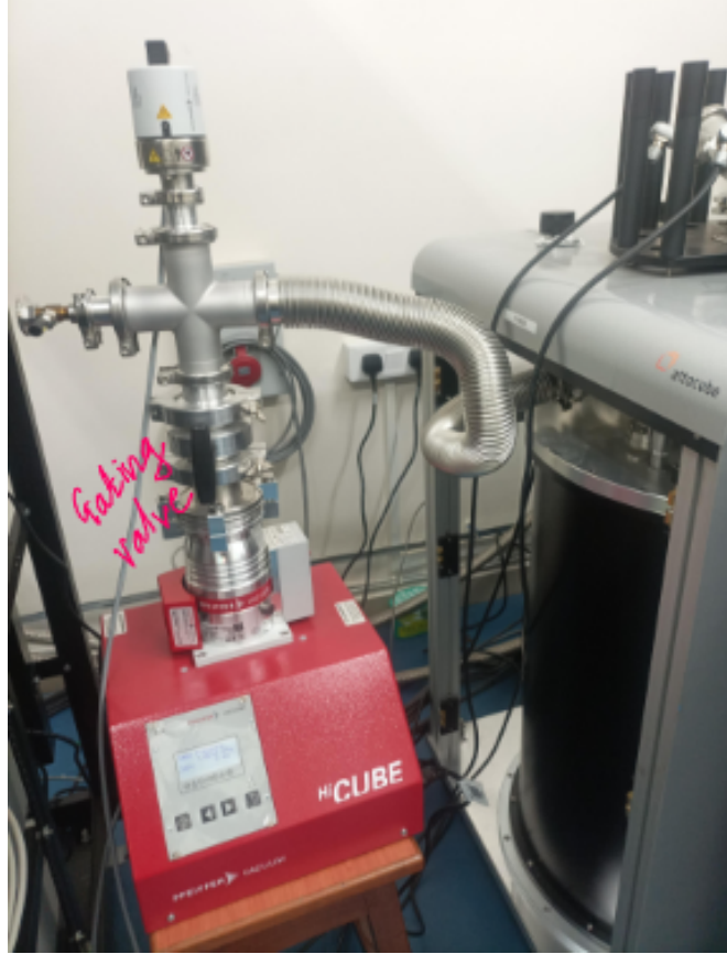
Figure 10: Suction pipe attached to Isolation chamber valve
