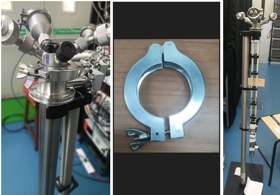
Figure 7: (left) Remove this lock; (middle) Lock; (right) Sample stick
