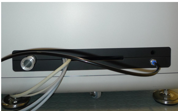
Figure 7: Preparing the attoDRY for inserting a microscope stick.
