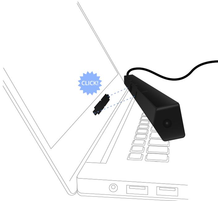
Figure 8. Place the mounting bracket on the bezel so that Tobii Pro Fusion is as close to the bottom of the screen as possible without covering the screen.
