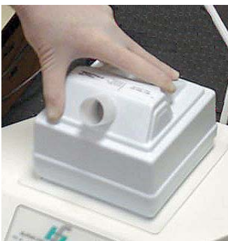
Figure 10-8 Seating the new filter
