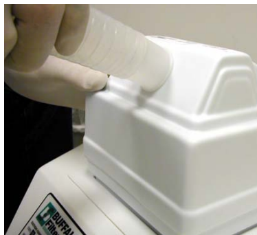
Figure 10-10 Connecting new tubing to the ULPA filter
