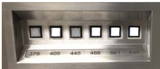
Figure 4-2 Laser power panel
