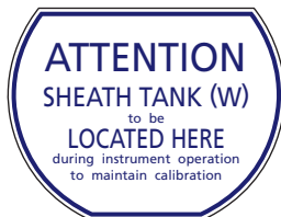
Figure 4-8 Sheath tank location label
