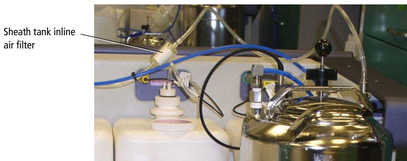
Figure 6-17 Inline air filter for sheath tank
