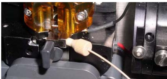
Figure 6-1 Closed-loop nozzle installed in flow cell
