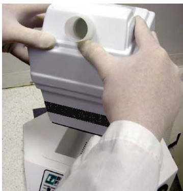
Figure 10-7 Inserting the new filter
